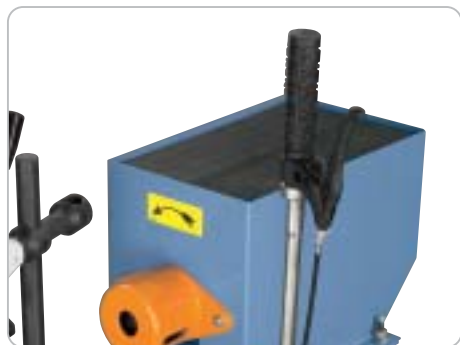
Motor cover can be used as tool storage
